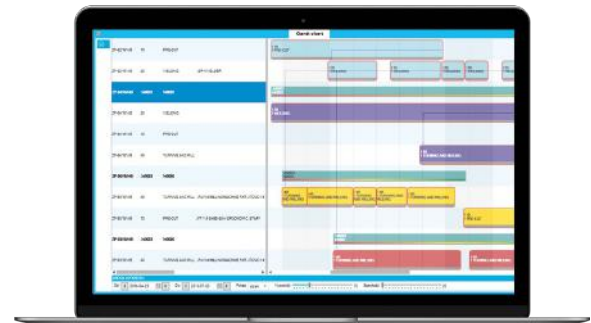
Production schedule can be visualised with the use of Gantta diagram, which clearly illustrates a progress of works and enables change of deadlines for planned activities.
